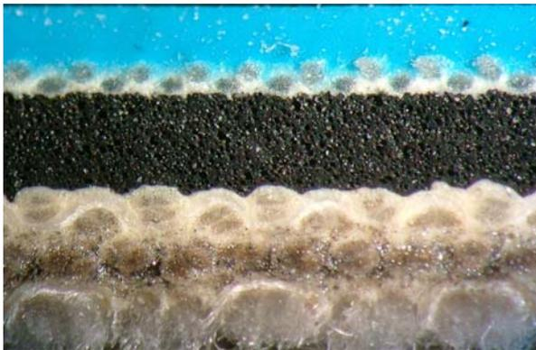
A typical compressive blanket with four plies. Please note the voids free structure and almost vitreous look reinforcement.
