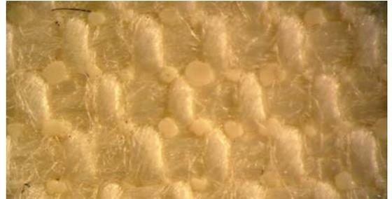
Carcass cloth surface showing excess rubber 'spots' from the first to the second ply gluing film.
